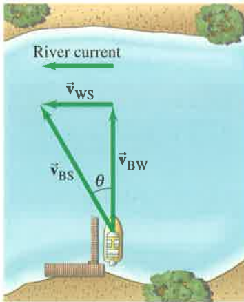
FIGURE 3-30 Example 3-12. A boat heading directly across a river whose current moves at 1.20 m/s.
